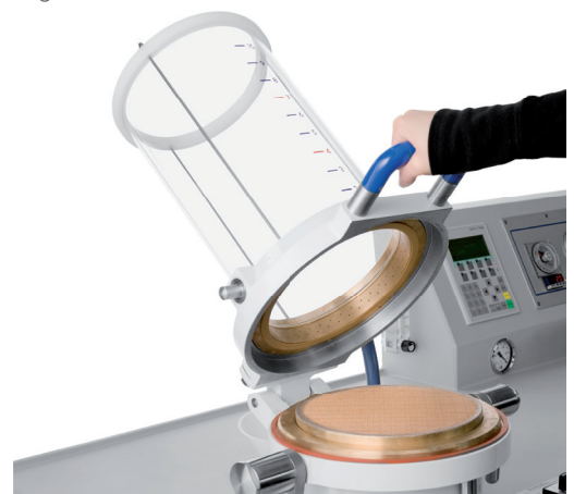
Opening the former column for taking out the hand-sheet
